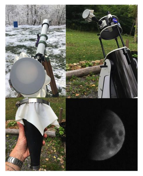
Sun Funnels in action! Starting clockwise from the bottom left, a standalone Sun Funnel; attached to a small refractor to observe the transit of Mercury in 2019; attached to a large telescope in preparation for evening lunar observing; projection of the Moon onto a funnel from a medium-size scope (5 inches).
